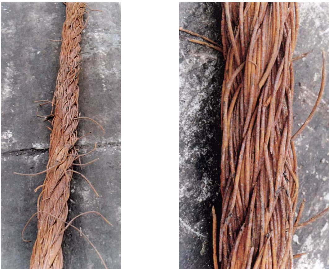
Figure 7 : Example of a six strand RHO lay mooring line removed from service which is believed to have experienced combined tension-torsion fatigue.
