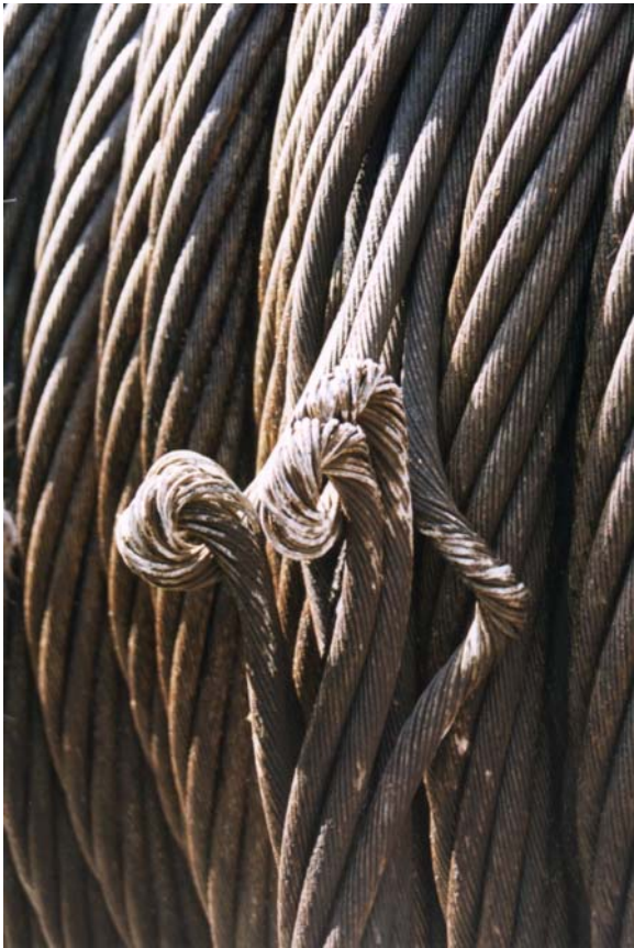
Figure 3 : Severe individual strand hockling in an 8 strand work wire.
