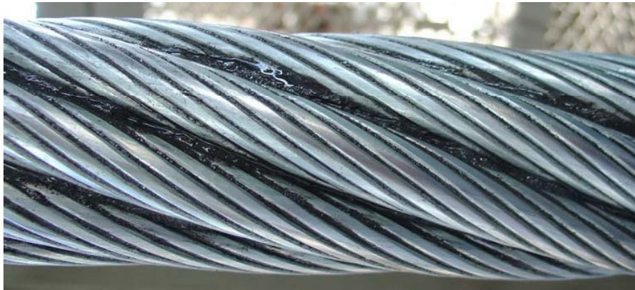
Figure 5b: Turboplast as-installed exterior.
