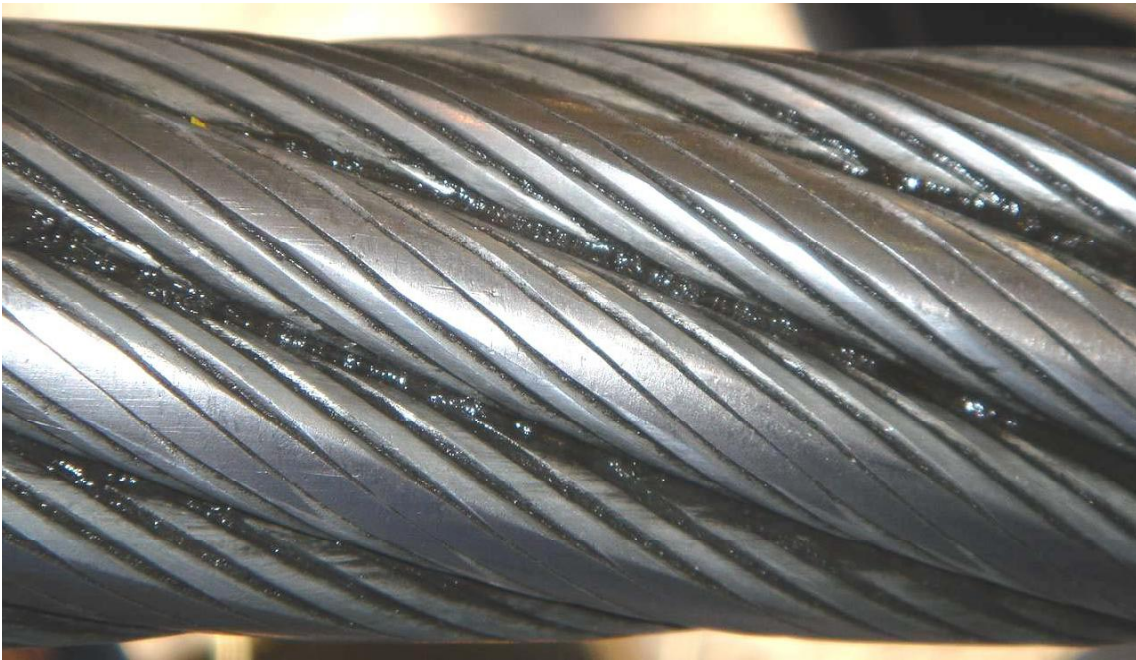
Figure 7: Typical layer crossover area plastic wear after circa 20,000 cycles.
