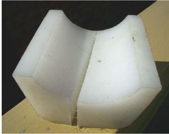
Figure 3: Polypropylene inserts as fitted to the rock winder headgear sheaves. These inserts were used for both the TSRs and the eight-strand ropes.
