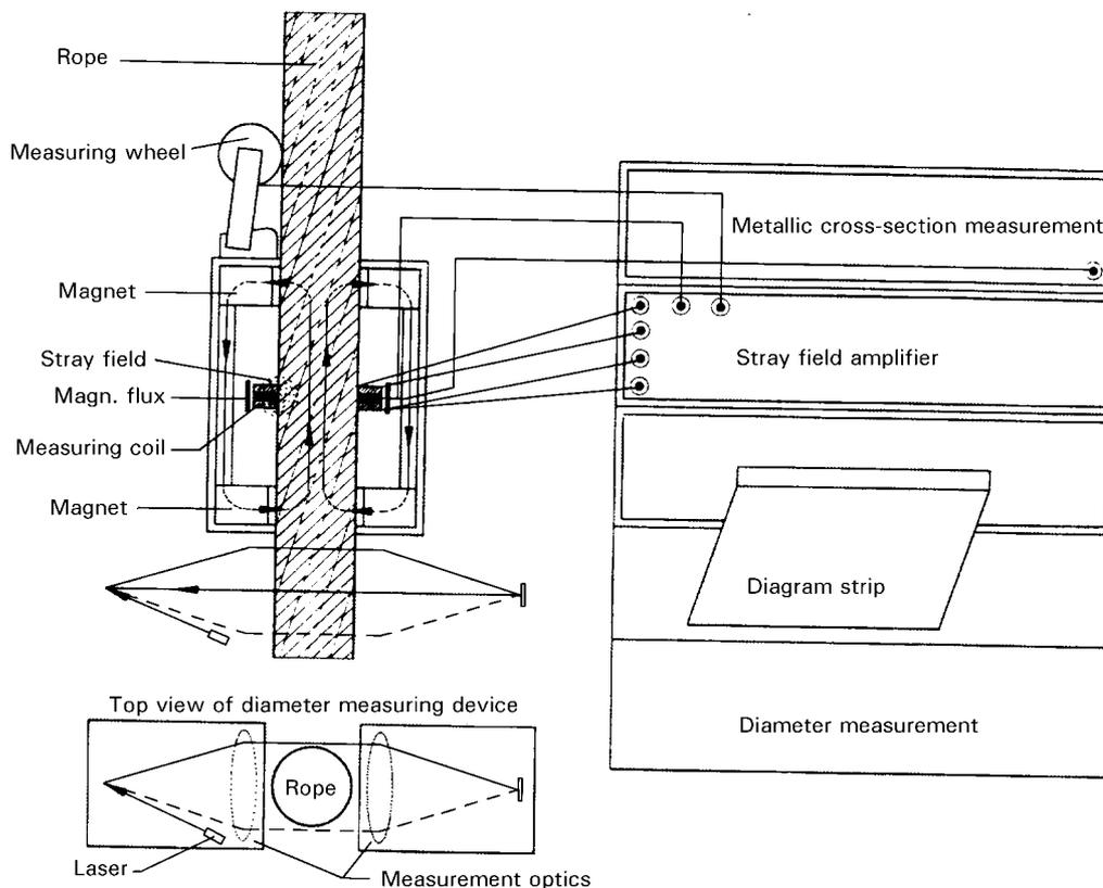
Figure 9 - Rope NDT system with three measurement parameters<sup>12</sup>.
