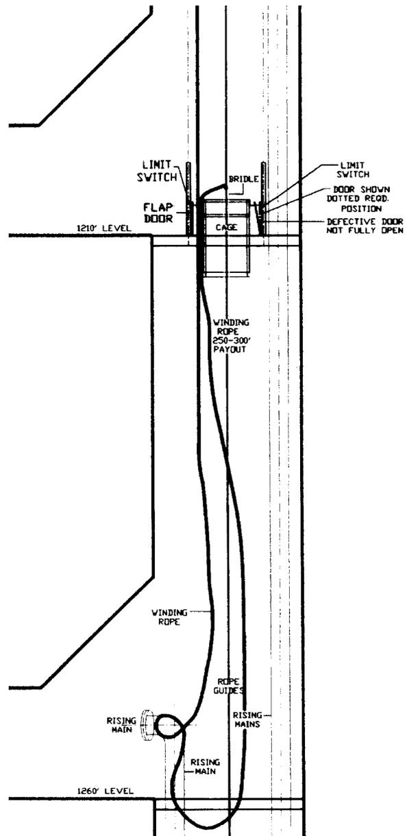
Figure 4 - VS1B cage held at the shaft door<sup>5</sup>, slack rope accident. See Table 1.
