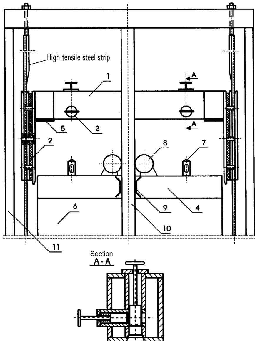
Figure 15 - Elevation of conveyance entering the HS2W-2 friction braking device<sup>21</sup>
