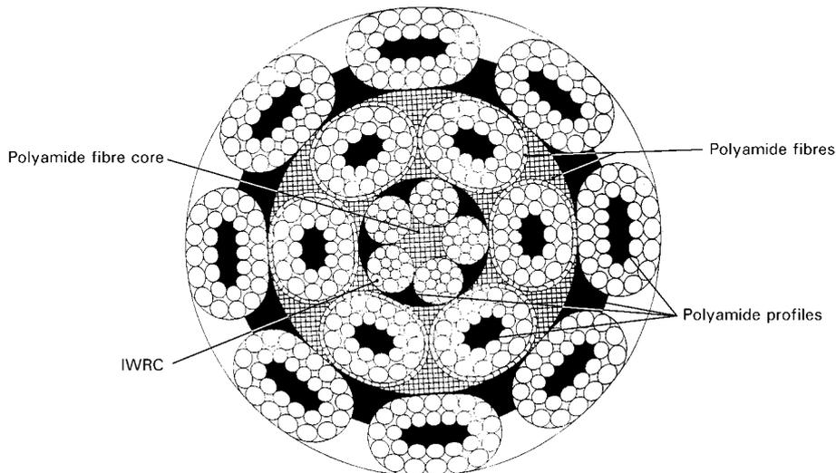
Figure 14 - Patented, three layer flattened strand rope construction<sup>16</sup>.
