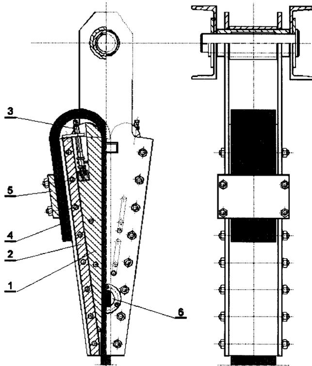
Figure 12 - The self locking wedge capel for SAG ropes<sup>15</sup>
