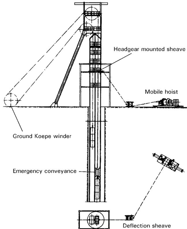
Figure 2 - A mobile emergency hoist installation<sup>1</sup> - original system.
