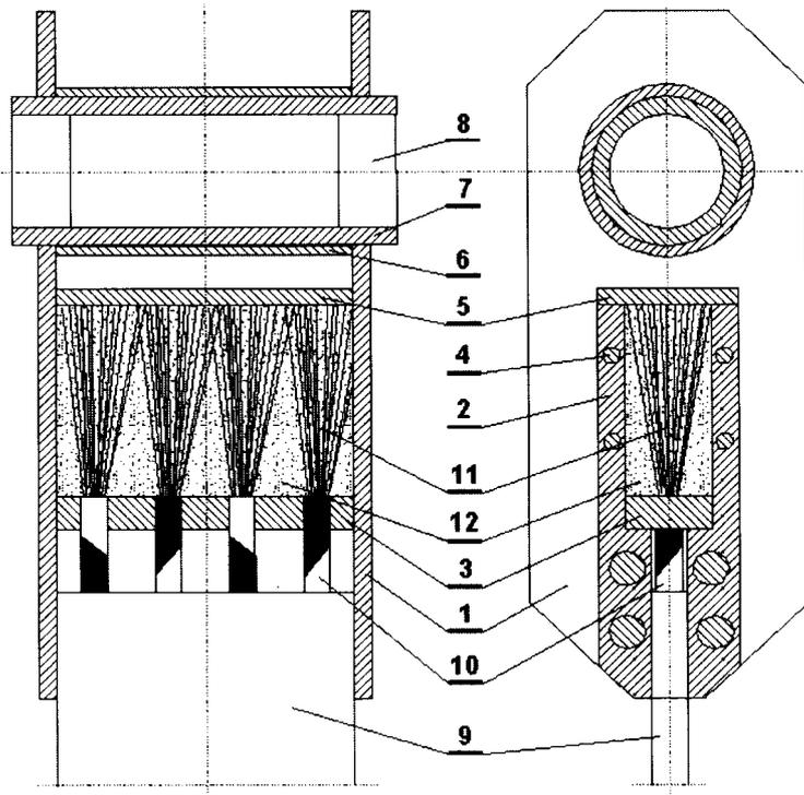
Figure 13 - The closed capel design for SAG ropes<sup>15</sup>
