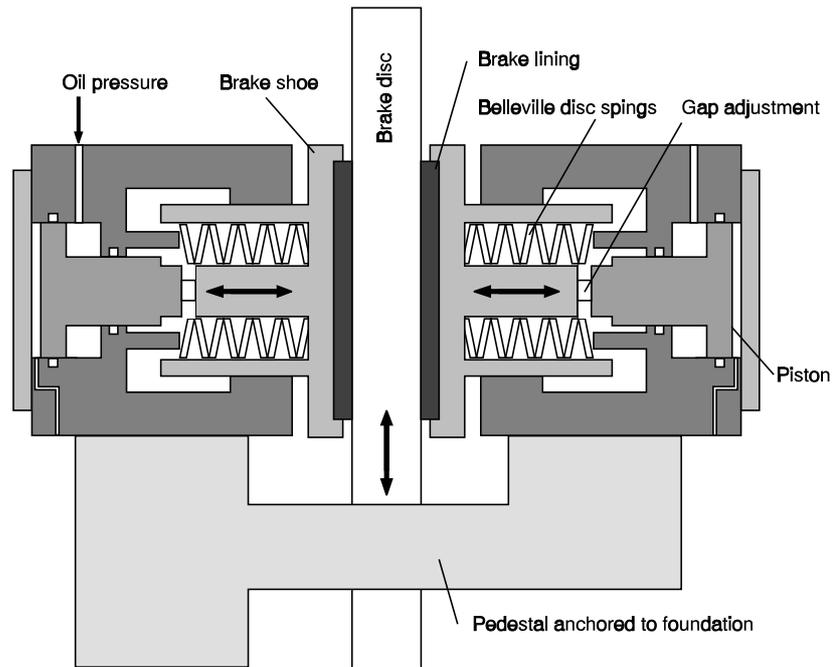
Figure 7 - Basic layout of disc brake calliper units, adapted from Brokenshire<sup>22</sup>.
