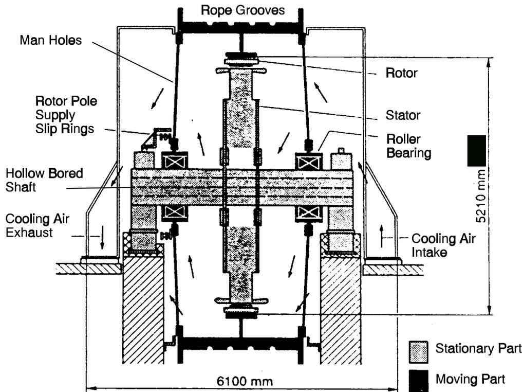
Figure 3 - Example of an integrated Koepe winder<sup>19</sup>.
