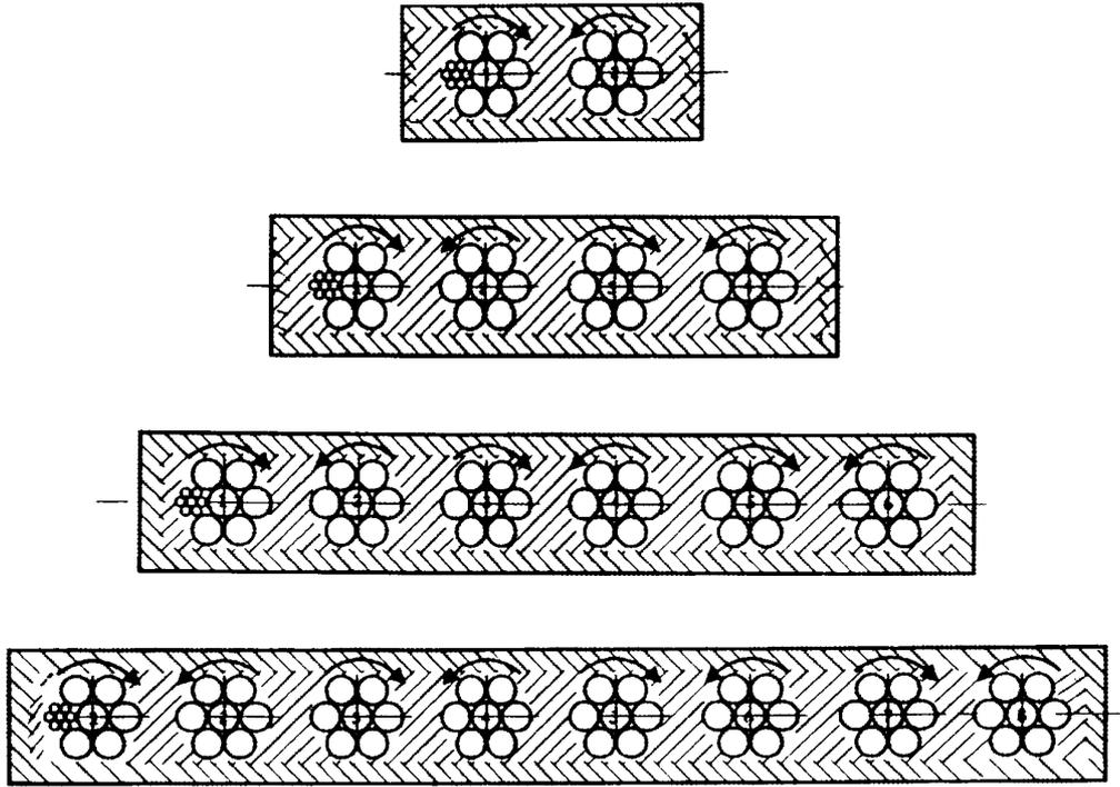
Figure 11 - Cross-section configurations of the SAG flat steel wire rubber balance ropes<sup>13</sup>.
